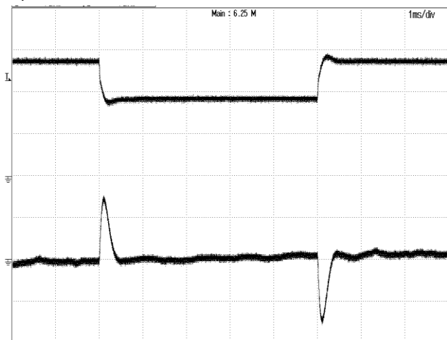
Figure 5: Output voltage response to step-change in load current (50%-75%-50% of full load; di/dt = 0.1A/\mu s ).
